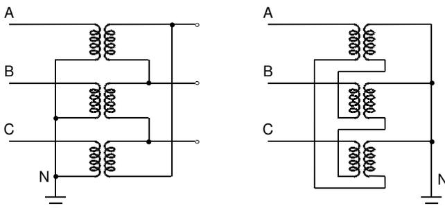
Fig. 5. Wye-delta (left) and Zig-Zag (right) grounding transformers
