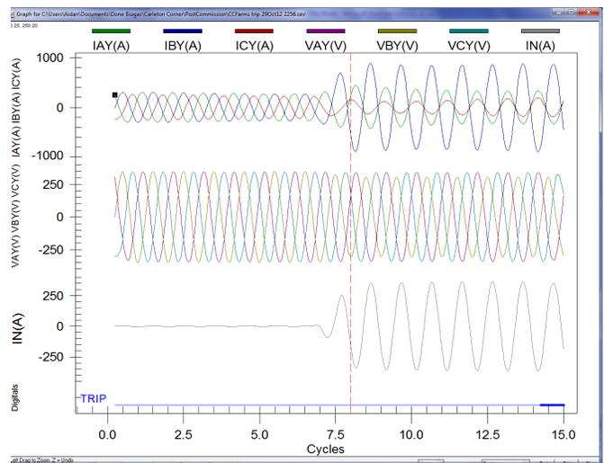
Fig. 7. Feeder ground fault (showing generator currents and voltages, and neutral current through the grounding transformer)
