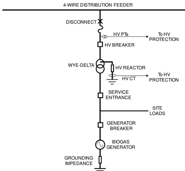
Fig. 4. Typical wye-delta transformer connection.
