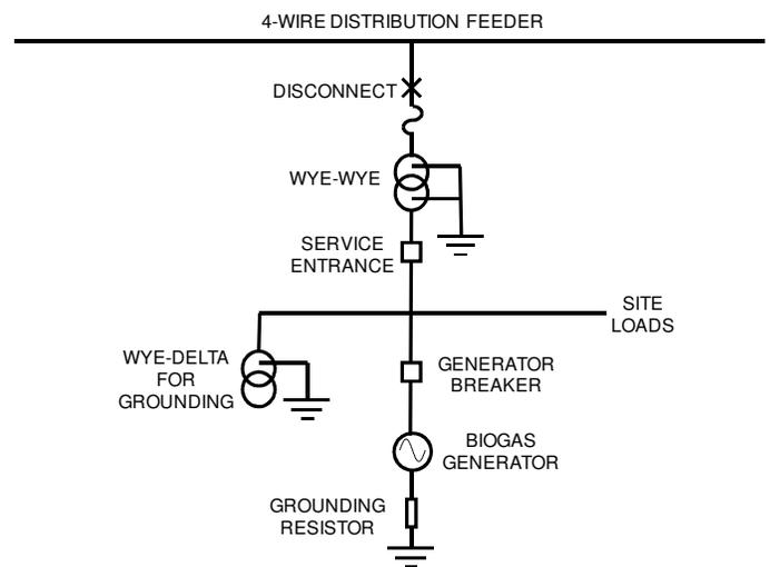
Fig. 6. Wye-wye transformation with LV grounding transformer
