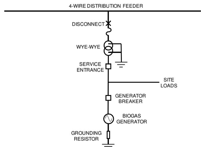
Fig. 3. Wye-wye transformation with impedance grounding.
