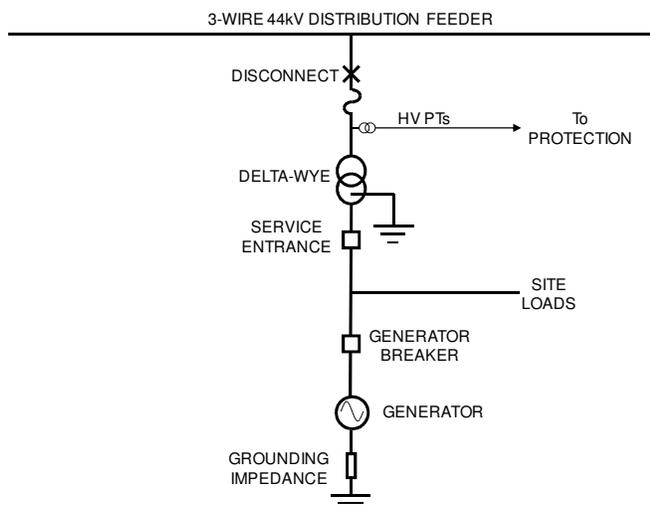
Fig. 1. Typical connection to 44kV 3-wire feeder.
