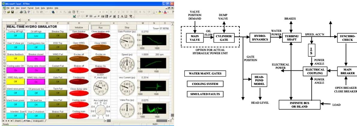
Figure 3.6: Real-time Hydro Simulator Tool (a) Interface and (b) Dynamic Model
