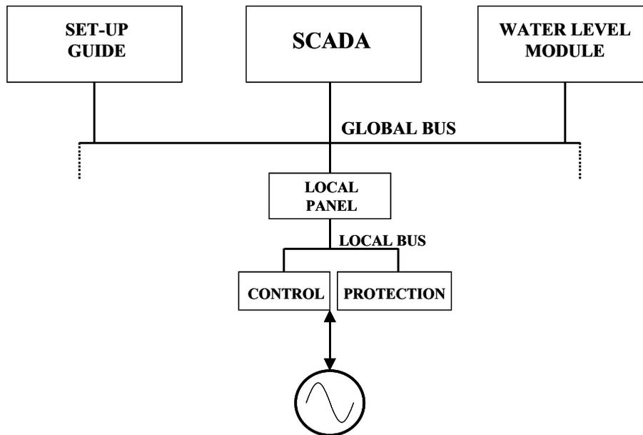
Figure 3.1: Equipment Structure for 2 MVA Hydro Generating Unit
