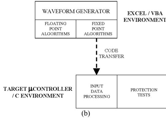
Using the simulation, measurement algorithms were prepared and verified taking into account appropriate sampling and analogue-to-digital conversion requirements. Algorithms were first prepared and verified using floating-point arithmetic, and then implemented fixed-point arithmetic in order to achieve the required computational speed whilst maintaining accuracy. Following verification, algorithms were converted to ‘C’ and copied across to the target micro-controller environment (Figure 3(b)).
