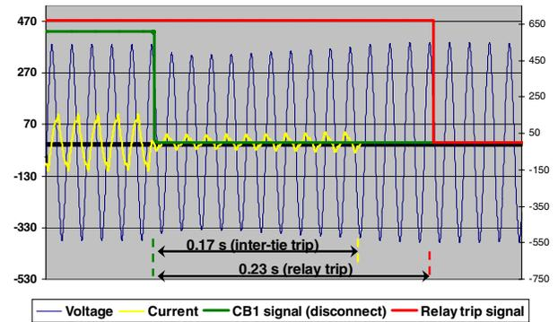
Fig. 9. Islanding case FT-6: 40Q relay tripped after the inter-tie CB tripping
