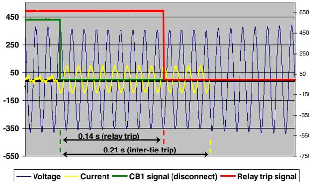
Fig. 8. Islanding case FT-1: 40Q relay tripped before the inter-tie CB tripping
