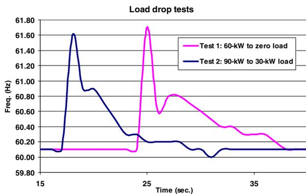
Fig. 7. Load drop tests at two different operating points
