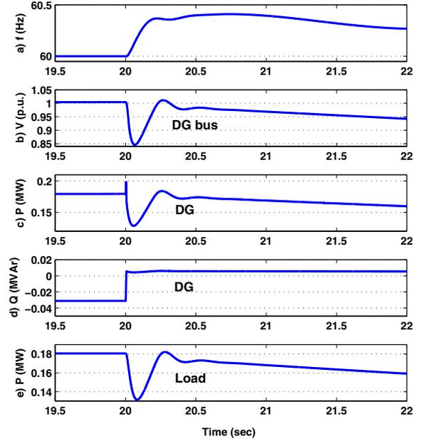
Fig. 5. Islanding at  $t=20$  s., zero load/generation imbalance (resistive load)
