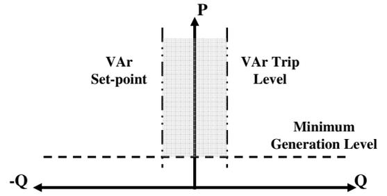
Fig. 1. Generator Operating and Trip Characteristic
