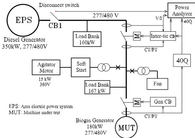
Fig. 6. Overview of electrical configuration of the field verification setup
