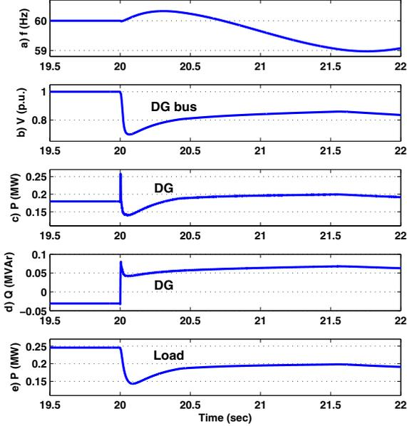
Fig. 4. Islanding at  $t=20$  s. for +25% power mismatch
