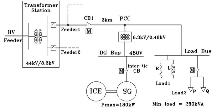
Fig. 2. One-line diagram of the rural feeder under study
