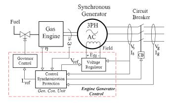
Fig. 3. Engine and Generator control systems
