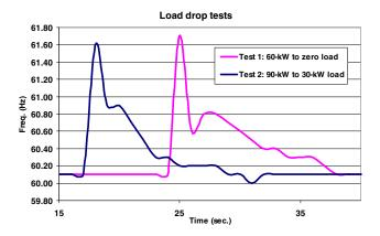
Fig. 7. Load drop tests at two different operating points
