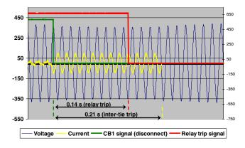
Fig. 8. Islanding case FT-1: 40Q relay tripped before the inter-tie CB tripping
