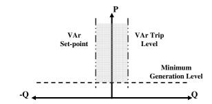
Fig. 1. Generator Operating and Trip Characteristic
