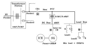
Fig. 2. One-line diagram of the rural feeder under study
