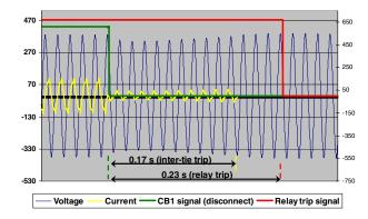
Fig. 9. Islanding case FT-6: 40Q relay tripped after the inter-tie CB tripping
