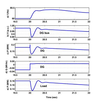
Fig. 5. Islanding at t=20 s., zero load/generation imbalance (resistive load)
